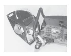
\* Replaces *DRY* Air Filter Canister When Using Water & Standard Water Kit (provided)
